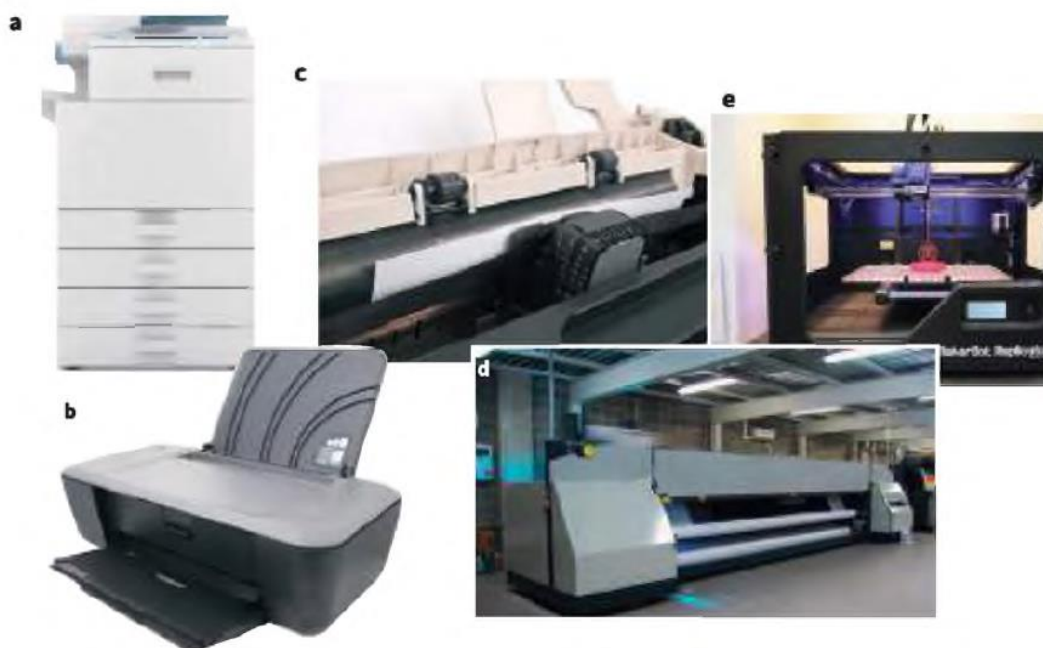
2.14-rasm. Printer turlari: (a) lazerli; (b) purkagichli; (c) matritsaii; (d) keng formatli va (e) 3D printer.
